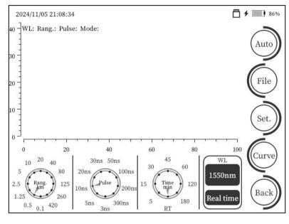
Setting method: On the main interface of the OTDR, click [Wave], and drag [1310nm], [1550nm] or [1310/1550nm] to the center frame.
