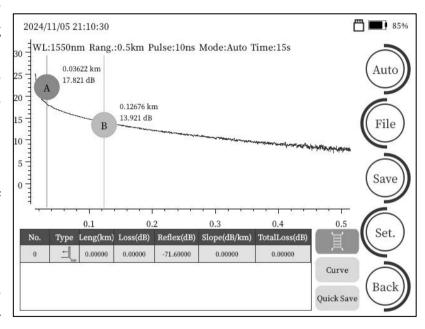
【 Auto Test 】 in automatic measurement mode. No other settings are required.
