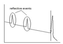
upward spike signal with a certain width. The width and amplitude of the spike are mainly determined by the pulse width used for the test and the reflection intensity that occurs.
