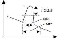
**Attenuation Blind Zone:** The shortest distance that OTDR goes through from detecting Fresnel reflection signal to normal testing backward Rayleigh scattering signal, that is, the phase cannot measure fusion loss due to adjacent large reflection.
