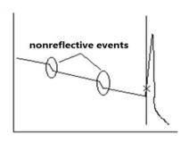
with a drop in energy on the OTDR test curve, and the magnitude of the drop indicates power loss.
