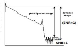
distance that OTDR can test under the condition of the maximum test pulse width provided by the instrument. Therefore, under the same link condition, the larger the dynamic range, the longer the distance of the optical fiber link that the instrument can test.
