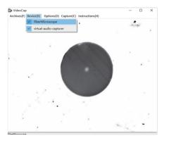
③ Insert the optical fiber end face to be detected into the detection interface, and then rotate the focus according to the display to a clear place. If the image is not in the center, the image can be adjusted to the middle of the screen by gently rotating the test joint.
